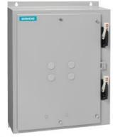
Duplex starter w/o alternator, Size 1, Three phase full voltage, Solid-state overload relay, OLR amp range 10-40A, 110V 50Hz / 120V 60Hz coil, Combination type, Two 30A circuit breakers, Enc NEMA type 4 painted steel, Water/dust tight for outdoors
