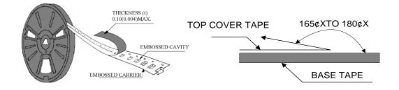
The peel off force of cover tape is 10 to 70 grams in the arrow direction.
