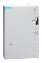
Non-reversing motor starter, Size 0, Three phase full voltage, Solid-state overload relay, OLR amp range 0.75-3.4A, 24VDC coil, Combination type, 30A fusible disconnect, 30A/250V fuse clip, Enclosure NEMA type 4/12, Water/dust tight for outdoors, Extra-wide enclosure
