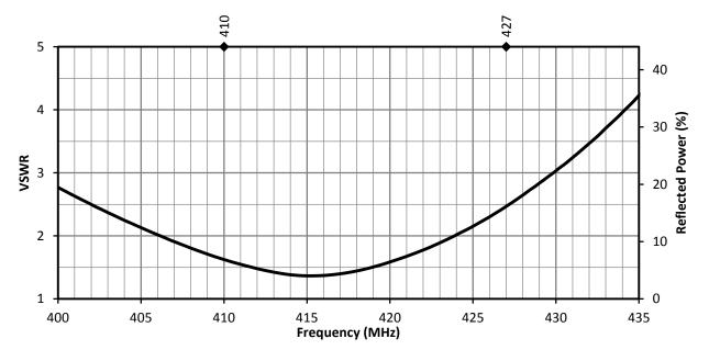
Figure 12. ANT-418-WRT VSWR, at Center of Ground Plane
