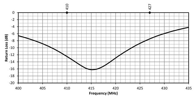
Figure 13 ANT-410-WRT Return Loss, at Center of Ground Plane
