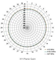
Figure 17. ANT-410-WRT Radiation Patterns, Center of Ground Plane
