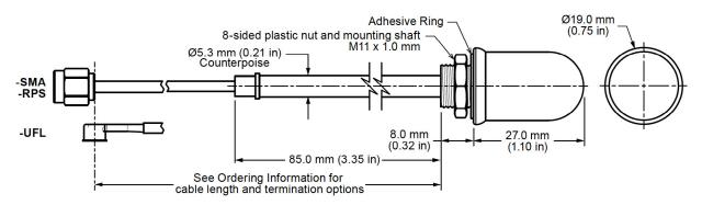
Figure 1. ANT-410-WRT-ccc Antenna Dimensions
