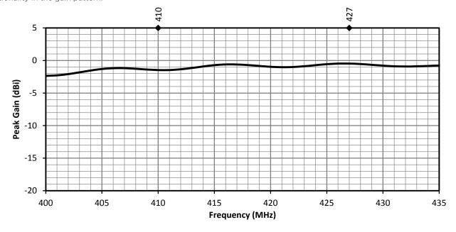
Figure 14. ANT-410-WRT Peak Gain, at Center of Ground Plane
