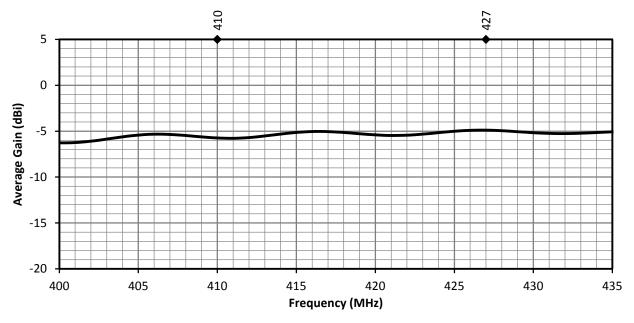
Figure 15. ANT-410-WRT Antenna Average Gain, at Center of Ground Plane
