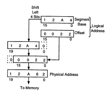
Figure 2. Two-Component Address
