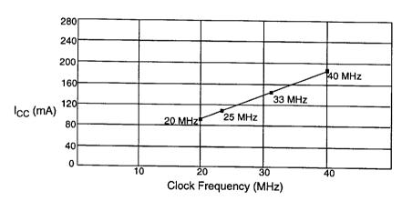
Figure 14. Typical I<sub>CC</sub> Versus Frequency for the Am186EM and Am188EM
