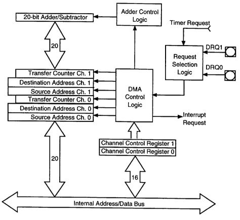
Figure 10. DMA Unit Block Diagram
