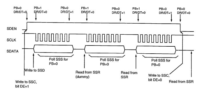
Figure 12. Synchronous Serial Interface Multiple Read
