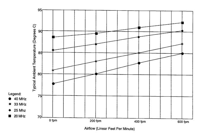
Figure 19. Typical Ambient Temperatures for PQFP with 4-Layer to 6-Layer Board
