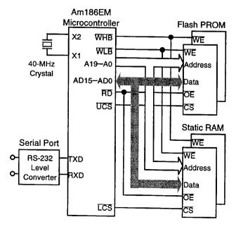
Figure 1. Example System Design
