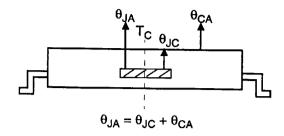
Figure 15. Thermal Resistance(°C/Watt)
