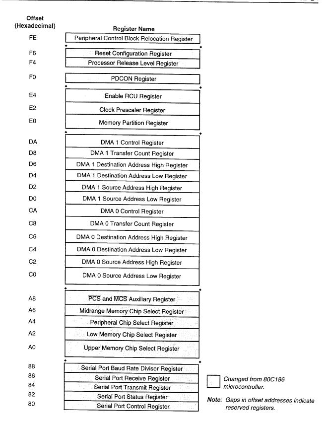
Figure 7. Peripheral Control Block Register Map
