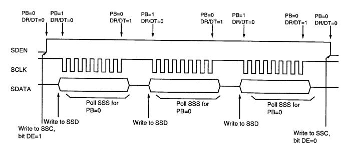
Figure 11. Synchronous Serial Interface Multiple Write
