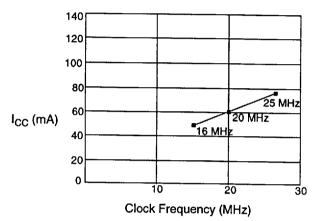
Figure 13. Typical I<sub>CC</sub> Versus Frequency for the Am186EMLV and Am188EMLV
