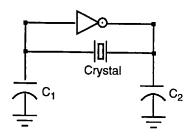
a. Inverting Amplifier Configuration
