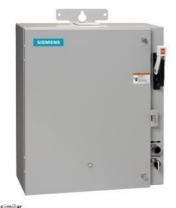
Pump control panel, Size 1, Three phase full voltage, Solid-state overload relay, OLR amp range 0.75-3.4A, 110-120/220-240VAC 60Hz coil, Standard type contactor, 3A circuit breaker, HOA Sel Sw. <(>&<)> Start P.B., Enclosure NEMA type 3/3R, Weather proof outdoor use
