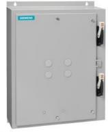
Duplex starter w/o alternator, Size 0, Three phase full voltage, Solid-state overload relay, OLR amp range 5.5-22A, 110V 50Hz / 120V 60Hz coil, Combination type, Two 25A circuit breakers, Enclosure NEMA type 12, Dust/drip proof for indoors
