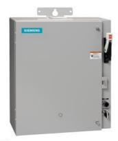
Pump control panel, Size 6, Three phase full voltage, Solid-state overload relay, OLR amp range 160-630A, 220-240V 50-60Hz/DC coil, Standard type contactor, 400A circuit breaker, HOA Sel Sw. <(>&<)> Start P.B., Enclosure NEMA type 3/3R, Weather proof outdoor use
