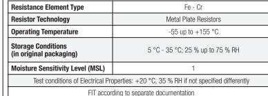
FIT according to separate documentation Component conform to REACh and RoHS requirements and standards
