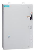
Non-reversing motor starter, Size 1, Three phase full voltage, Solid-state overload relay, OLR amp range 0.75-3.4A, Combination type, 30A fusible disconnect, 30A/600V fuse clip, Enclosure NEMA type 4/12, Water/dust tight for outdoors, Extra-wide enclosure
