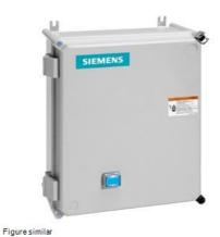
Non-reversing motor starter, Size 1, Three phase full voltage, Solid-state overload relay, OLR amp range 10-40A, 110V 50Hz / 120V 60Hz coil, Non-combination type, Enclosure type 4X fiberglass, Water/dust tight noncorrosive, Standard width enclosure
