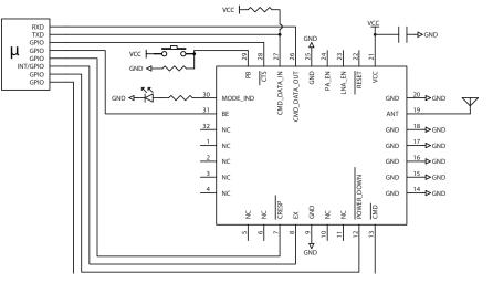
Figure 107: HumPRO<sup>™</sup> Series Transceiver Basic Application Circuit
