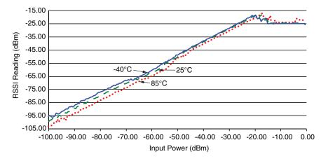
Figure 13: HumPRO<sup>™</sup> Series Transceiver RSSI Voltage vs. Input Power - HUM-868-PRO
