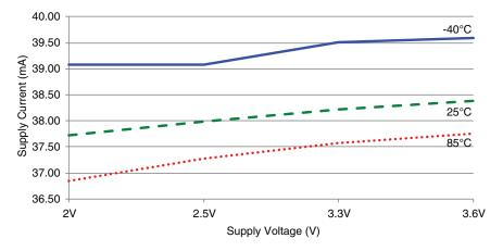
Figure 7: HumPRO<sup>™</sup> Series Transceiver TX Current vs. Supply Voltage at Max Power - HUM-868-PRO
