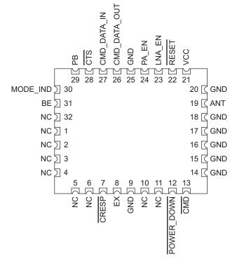
Figure 14: HumPRO<sup>™</sup> Series Transceiver Pin Assignments (Top View)
