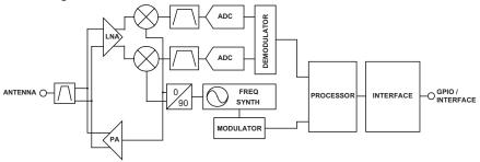
Figure 20: HumPRO<sup>™</sup> Series Transceiver RF Section Block Diagram
