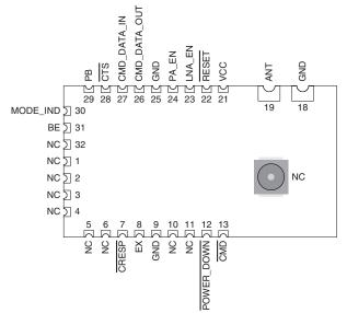
Figure 16: HumPRO<sup>™</sup> Series Transceiver Encapsulated Version Pin Assignments - Castellation Connection (Top View)
