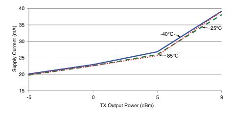
Figure 6: HumPRO<sup>™</sup> Series Transceiver Average Current vs. Transmitter Output Power at 2.5V - HUM-868-PRO
