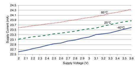
Figure 10: HumPRO<sup>™</sup> Series Transceiver RX Scan Current vs. Supply Voltage, 9.6kbps - HUM-868-PRO
