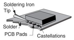
Figure 115: Soldering Technique
