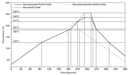
Figure 117: Maximum Reflow Temperature Profile
