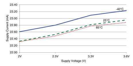
Figure 9: HumPRO<sup>™</sup> Series Transceiver TX Current vs. Supply Voltage at 0dBm - HUM-868-PRO
