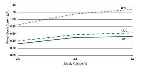
Figure 11: HumPRO<sup>™</sup> Series Transceiver Standby Current Consumption vs. Supply Voltage - HUM-868-PRO
