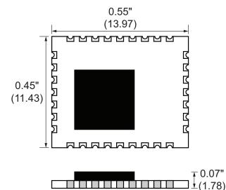
Figure 18: HumPRO<sup>™</sup> Series Transceiver Dimensions
