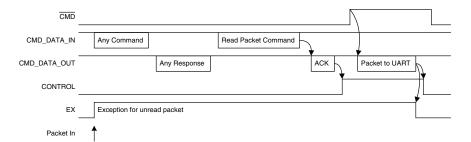
Figure 23: HumPRO<sup>™</sup> Series Transceiver Received Packet Transfer Cycle
