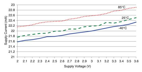
Figure 12: HumPRO<sup>™</sup> Series Transceiver RX Scan Current vs. Supply Voltage, 115.2kbps - HUM-868-PRO
