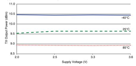
Figure 5: HumPRO<sup>™</sup> Series Transceiver Max Output Power vs. Supply Voltage - HUM-868-PRO
