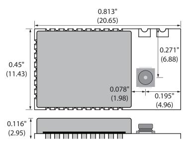
Figure 19: HumPRO<sup>™</sup> Series Transceiver Encapsulated Version Dimensions
