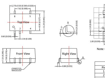
Note: Unit: mm[inch] Pin section tolerances: ±0.10mm[± 0.004inch] General tolerances: ±0.25mm[ ±0.010inch]
