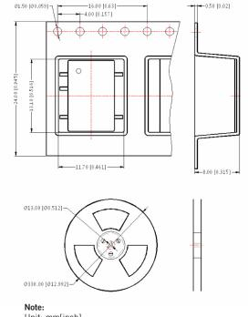
Note: Unit: mm[inch] General tolerances: 0.5mm[ 0.020inch] Devices per reel quantity: 500pcs
