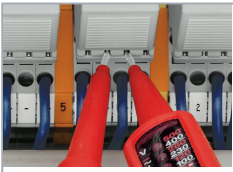
Function testing via touch-proof test slots
