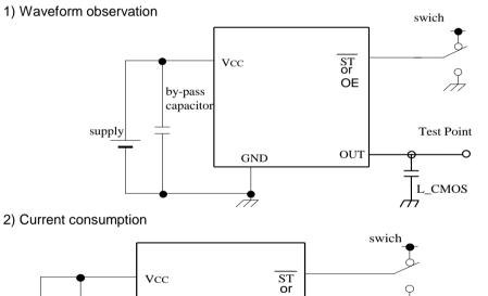
\*Current consumption under the disable function should be = GND.
