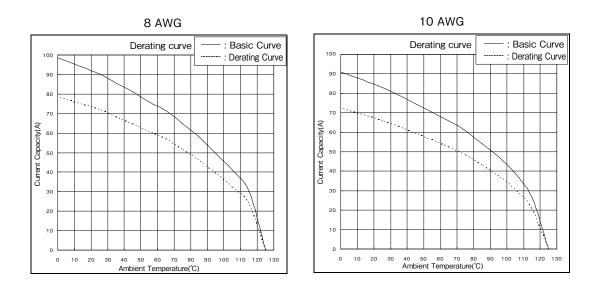
Note 1 : The derating curve is a curve is derived by multiplying the basic curve by the derating factor of 0.8.
