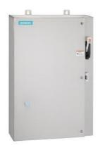
Non-reversing motor starter, Size 3, Three phase full voltage, Solid-state overload relay, OLR amp range 25-100A, Combination type, 125A circuit breaker, Encl NEMA type 4X 316 S-Steel, Water/dust tight noncorrosive, Extra-wide enclosure
