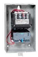
Non-reversing motor starter, Size 00, Three phase full voltage, Solid-state overload relay, OLR amp range 3-12A, 24VDC coil, Non-combination type, Enclosure type 1, Indoor general purpose use, Standard width enclosure
