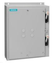
Duplex starter w/o alternator Size 1 Three phase full voltage Solid-state overload relay OLR amp range 0.25-1A 110VAC 50Hz / 120VAC 60Hz Coil Combination type Two 30A disconnect switches Enclosure NEMA type 4/12 Water/dust tight weather proof
