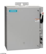
Pump control panel, Size 2, Three phase full voltage, Solid-state overload relay, OLR amp range 13-52A, 24VAC 50-60Hz coil, Standard type contactor, 50A circuit breaker, HOA Sel Sw. <(>&<)> Start P.B., Enclosure NEMA type 3/3R, Weather proof outdoor use
