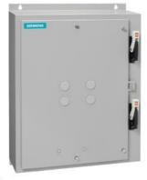
Duplex starter w/o alternator, Size 4, Three phase full voltage, Solid-state overload relay, OLR amp range 50-200A, 240V 50Hz / 277V 60Hz coil, Combination type, Two 150A circuit breakers, Encl NEMA type 4X 304 S-Steel, Water/dust tight noncorrosive
