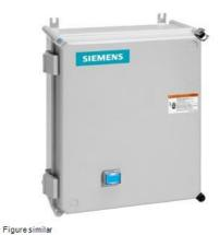
Non-reversing motor starter, Size 3, Three phase full voltage, Solid-state overload relay, OLR amp range 25-100A, Non-combination type, Enclosure type 4X fiberglass, Water/dust tight noncorrosive, Standard width enclosure
