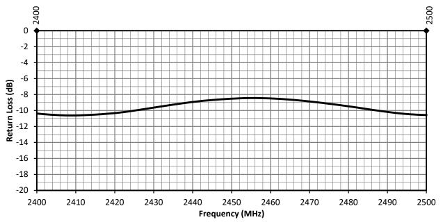
Figure 5. ANT-2.4-MMG2-SMA Antenna Return Loss on Ground Plane
