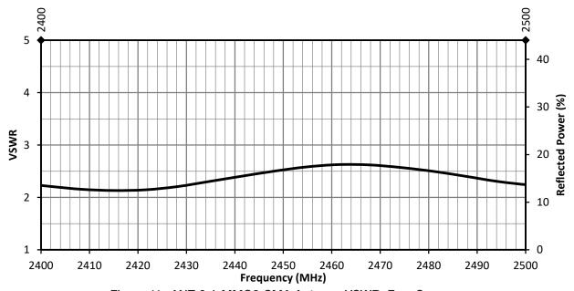
Figure 11. ANT-2.4-MMG2-SMA Antenna VSWR, Free Space
