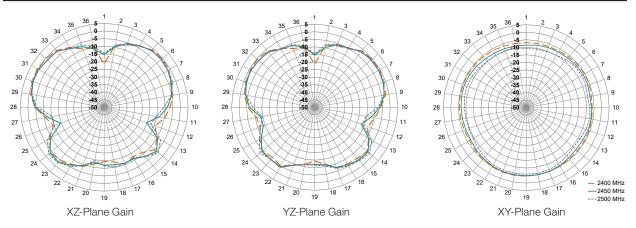
Figure 16. Radiation Patterns for ANT-2.4-MMG2-SMA Antenna, Free Space
