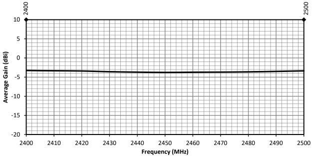
Figure 7. ANT-2.4-MMG2-SMA Antenna Average Gain on Ground Plane
