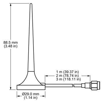
Figure 1. ANT-2.4-MMG2-SMA Series Antenna Dimensions
