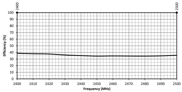
Figure 15. ANT-2.4-MMG2-SMA Antenna Radiation Efficiency, Free Space
