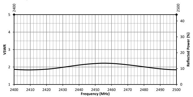
Figure 4. ANT-2.4-MMG2-SMA Antenna VSWR on Ground Plane
