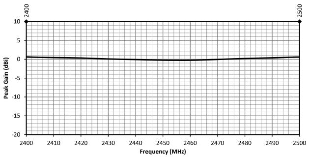
Figure 13. ANT-2.4-MMG2-SMA Antenna Peak Gain, Free Space
