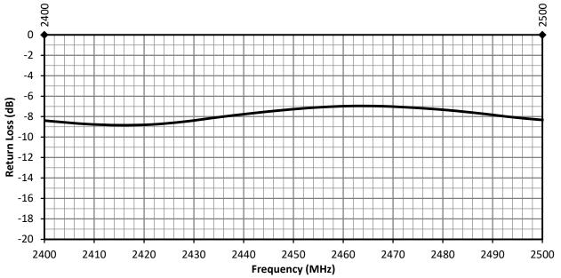
Figure 12. ANT-2.4-MMG2-SMA Antenna Return Loss, Free Space
