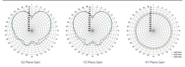
Figure 9. Radiation Patterns for ANT-2.4-MMG2-SMA Antenna on Ground Plane
