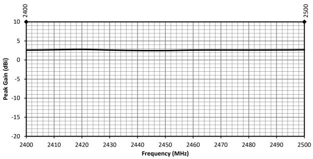
Figure 6. ANT-2.4-MMG2-SMA Antenna Peak Gain on Ground Plane
