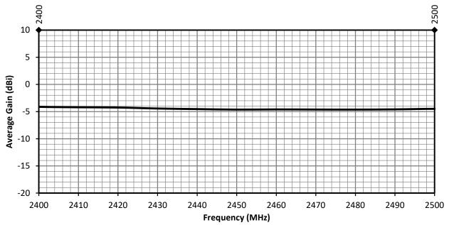
Figure 14. ANT-2.4-MMG2-SMA Antenna Average Gain, Free Space
