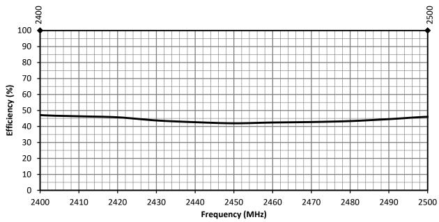
Figure 8. ANT-2.4-MMG2-SMA Antenna Radiation Efficiency on Ground Plane
