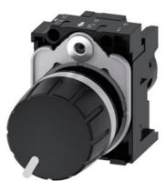
Potentiometer, compact, 22 mm, round, plastic, black, 1k ohm, with holder, screw terminal, with laser labeling, upper case
