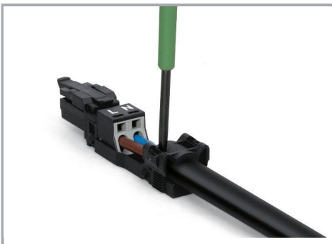
Push down strain relief clamp with 2.5 mm screwdriver alternately on both sides.
