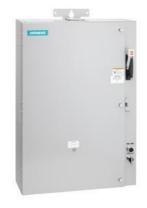
Pump control panel, Size 3, Three phase full voltage, Solid-state overload relay, OLR amp range 25-100A, 110-120/220-240VAC 60Hz coil, Standard type contactor, 100A fusible disconnect, 100A/250V fuse clip, HOA Sel Sw. <(>&<)> Start P.B., Enclosure NEMA type 3/3R, Weather proof outdoor use
