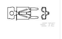
TE Part #63968-1 FASTON 205/250 LIF PCB MOUNTED TPBR
