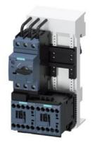
FUSELESS LOAD FEEDER REVERSING OPERATION, AC 400V, S00 4.5...6.3A, AC 110/120V 50/60HZ SCREW TERMINAL FOR BUSBAR SYSTEMS 60MM TYPE OF ASSIGNMENT 1,IQ = 150KA 1NC (CONTACTOR)
