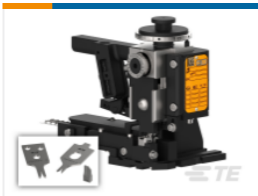
TE Part # 7-2151020-1 OCEAN_2.0_APPLICATOR-S-055F062O
