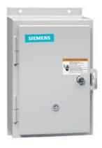
Reversing motor starter, Size 0, Three phase full voltage, Solid-state overload relay, OLR amp range 0.25-1A, 110V 50Hz / 120V 60Hz coil, Non-combination type, Enclosure type 12, Dust/drip proof for indoors, Standard width enclosure
