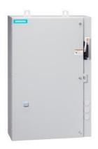
Non-reversing motor starter, Size 1, Three phase full voltage, Solid-state overload relay, OLR amp range 0.25-1A, Combination type, 30A fusible disconnect, 30A/250V fuse clip, Enclosure NEMA type 4/12, Water/dust tight for outdoors, Extra-wide enclosure
