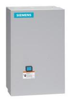
Non-reversing motor starter, Size 2 1/2, Three phase full voltage, Amb. compensate bimetal OLR, Contactor amp rating 60A, 240V 50Hz / 277V 60Hz coil, Non-combination type, Enclosure type 1, Indoor general purpose use
