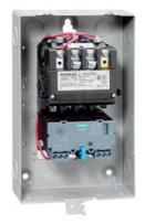
Non-reversing motor starter, Size 1, Three phase full voltage, Solid-state overload relay, OLR amp range 5.5-22A, 110V 50Hz / 120V 60Hz coil, Non-combination type, Enclosure type 1, Indoor general purpose use, Extra-wide enclosure
