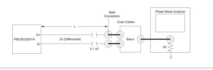
Figure 5. Test Setup for PI6CB332001A Additive Phase Jitter Measurement
