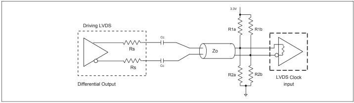
Figure 4. Differential Output Driving LVDS
