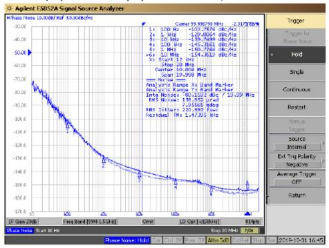
156.25MHz input phase noise vs output phase noise. Additive jitter<sup>1</sup> 51fs.
