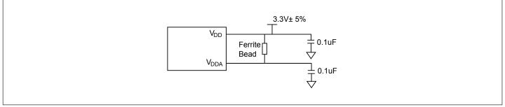
Figure 6. Power Supply Filter
