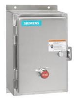
Non-reversing motor starter, Size 3 1/2, Three phase full voltage, Amb. compensate bimetal OLR, Contactor amp rating 115A, 24VDC coil, Non-combination type, Encl. type 4X 304 S. Steel, Water/dust tight noncorrosive
