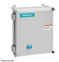
Non-reversing motor starter, Size 1, Single phase full voltage, Solid-state overload relay, OLR amp range 3-12A, 110V 50Hz / 120V 60Hz coil, Noncombination type, Enclosure type 4X fiberglass, Water/dust tight noncorrosive, Standard width enclosure
