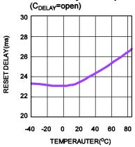
Reset Delay vs.Temperature
