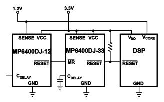
Figure 5— MP6400 Family Monitoring Multiple System Voltages
