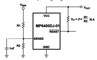
Figure 4—MP6400DJ-01 Monitoring a User-Defined Voltage
