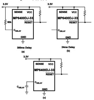
Figure 7—Programmable Configurations to the Reset Delay Time
