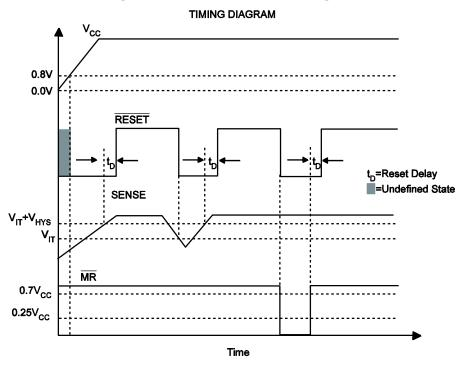
Figure 2—MP6400 Timing Diagram
