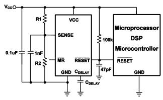
Figure 3—Typical Application of MP6400 with Microprocessor
