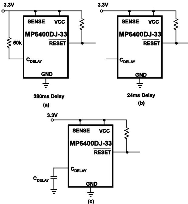
**Figure 7—Programmable Configurations to the Reset Delay Time**
