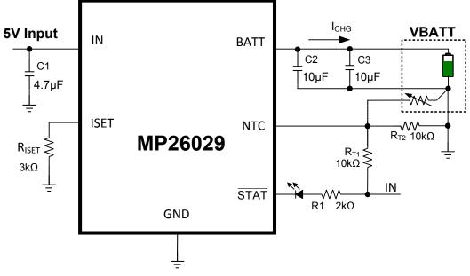
Figure 8: MP26029 Typical Application Circuit with 5V Input
