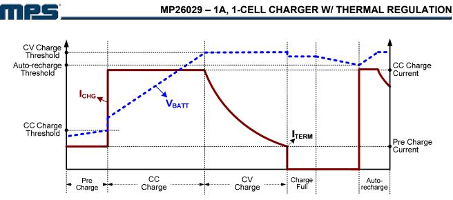
Figure 2: Battery Charge Profile
