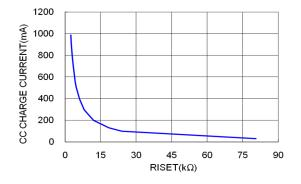
Figure 7: Charge Current vs. RISET Resistance
