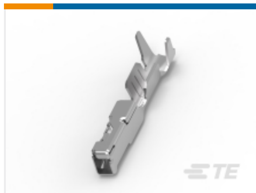
TE Part #2098762-4 Contact,female0.64, 22 AWG, CuNiSi, Sn
