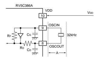
Typical externally-equipped element X'tal: 32.768 kHz (R1= $30 k\Omega$  TYP.)
