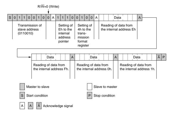
3) The third method to reading data from the internal register is to start reading immediately after writing to the slave address and the  $R/\overline{W}$  bit. Since the internal address pointer is set to Fh by default as described in 1), this method is only effective when reading is started from the internal address Fh.
