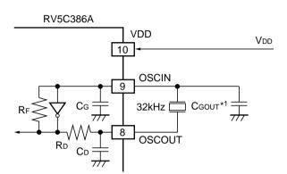
\*1) The CGOUT should have a capacitance ranging from 0 to 15pF.
