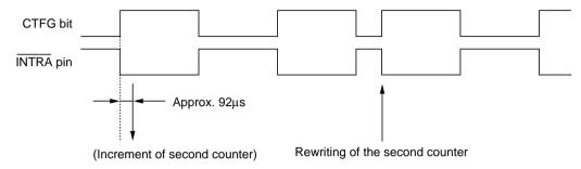
\*) In the pulse mode, the increment of the second counter is delayed by approximately 92µs from the falling edge of clock pulses. Consequently, time readings immediately after the falling edge of clock pulses may appear to lag behind the time counts of the real-time clocks by approximately 1 second. Rewriting the second counter will reset the other time counters of less than 1 second, driving the INTRA pin low.
