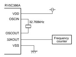
$X'tal:32.768kHz $$ (R_1=30k\Omega\ TYP.)$ (Cl=6pF to 8pF)$
