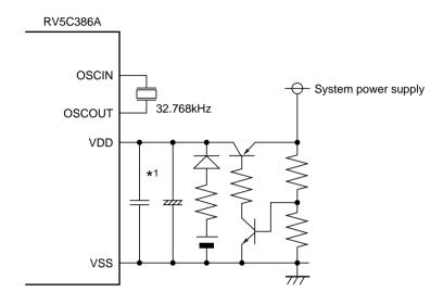
\*1) Install bypass capacitors for high-frequency and low-frequency applications in parallel in close vicinity to the RV5C386A.
