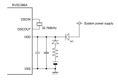
\*1) When using an OR diode as a power supply for the RV5C386A, ensure that voltage exceeding the absolute maximum rating of VDD +0.3 volts is not applied the 32KOUT pin.
