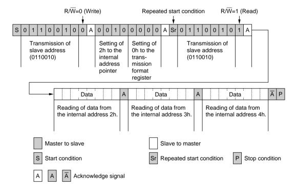
2) The second method to reading data from the internal register is to start reading immediately after writing to the internal address pointer and the transmission format register. Although this method is not based on the I<sup>2</sup>C bus standard in a strict sense it still effective to shorten read time to ease load to the master. Set 4h to the transmission format register when this method is used.
