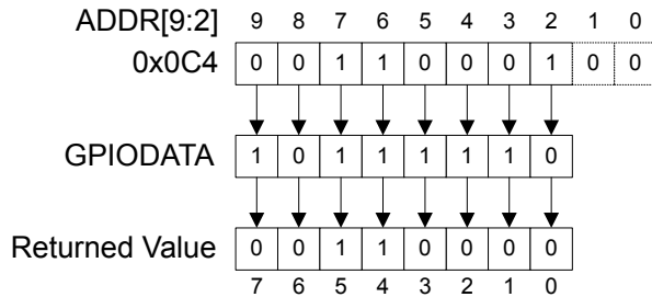
Figure 8-3. GPIO DATA Read Example
