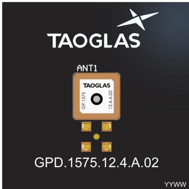
Top Side (GP.1575.12.4.A.02 placement on 50x50mm PCB)
