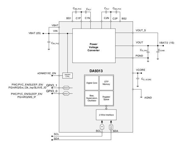
Figure 3: Functional Block Diagram Standalone (I<sup>2</sup>C Connected)
