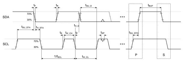
Figure 6: I<sup>2</sup>C Bus Timing
