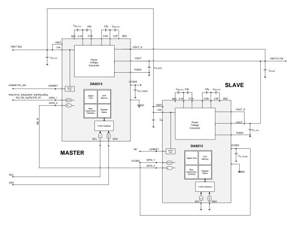
Figure 4: Functional Block Diagram Master/Slave Operation (I<sup>2</sup>C Connected)
