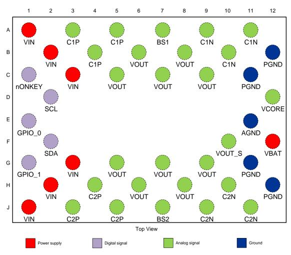
**Figure 5: Connection Diagram**
