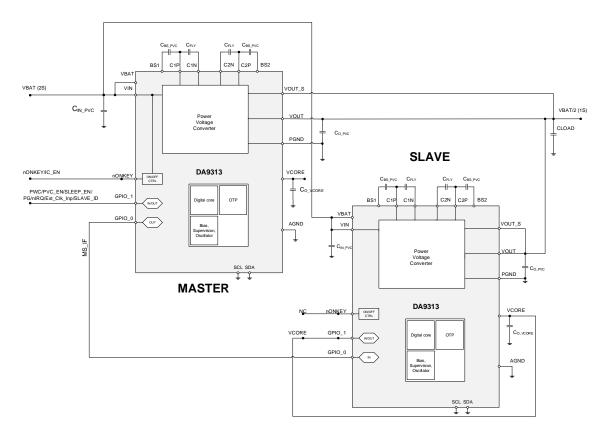
Figure 2: Functional Block Diagram Master/Slave Operation (I<sup>2</sup>C Not Connected)
