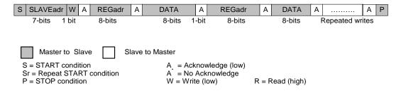
Figure 20: I<sup>2</sup>C Repeated Write (SDA Line)
