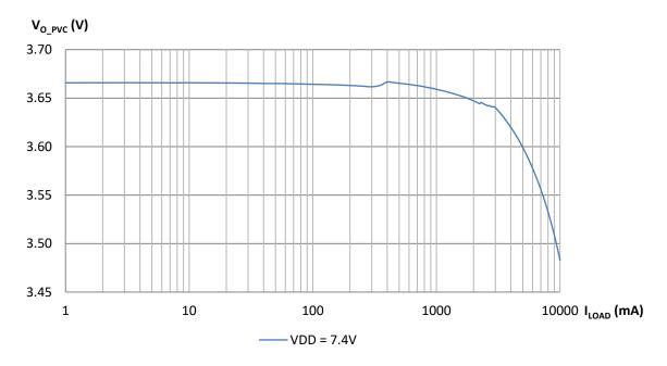
Figure 9: DA9313 Output Voltage Drop Automatic Mode Standalone
