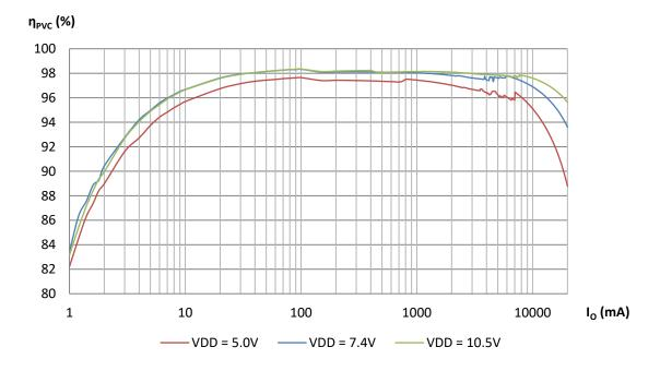
Figure 10: DA9313 Efficiency Automatic Mode Master/Slave
