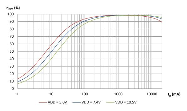
Figure 11: DA9313 Efficiency Fixed Frequency Mode Master/Slave
