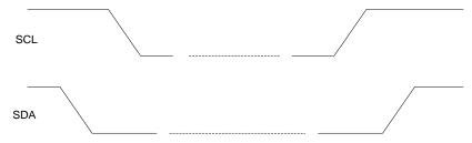
Figure 15: Timing of I<sup>2</sup>C START and STOP Condition
