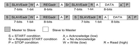
Figure 17: I<sup>2</sup>C Byte Read (SDA Line)
