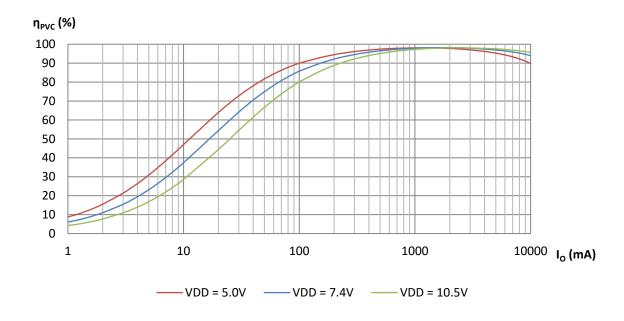
Figure 8: DA9313 Efficiency Fixed Frequency Mode Standalone
