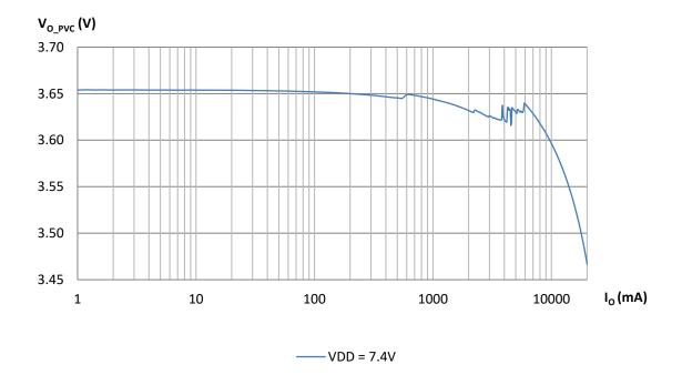
Figure 12: DA9313 Output Voltage Drop Automatic Mode Master/Slave
