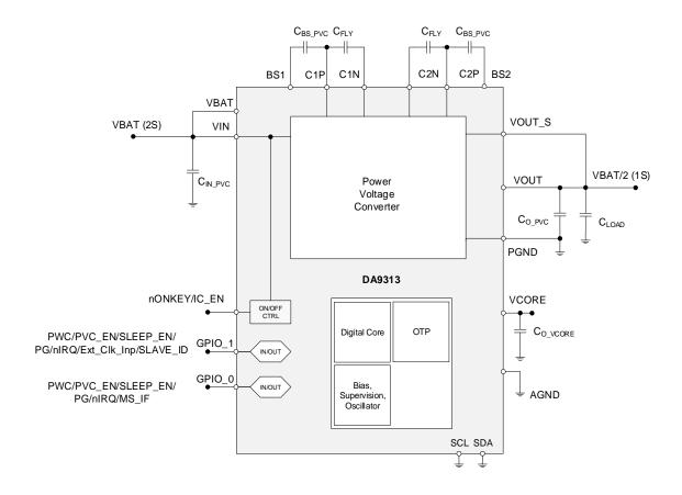
Figure 1: Functional Block Diagram Standalone (I<sup>2</sup>C Not Connected)
