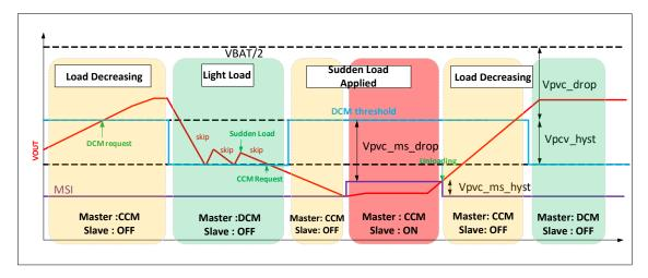
Figure 13: Master Slave Timing in Automatic Frequency Mode
