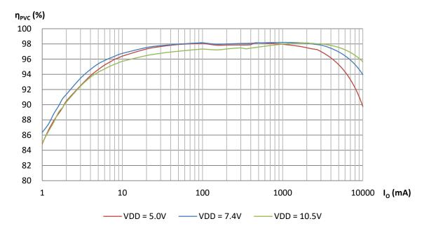
Figure 7: DA9313 Efficiency Automatic Mode Standalone
