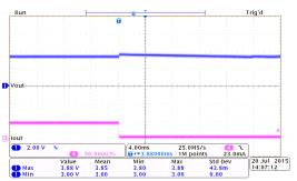
Load Transient Response: HT7333-2 (V<sub>IN</sub>=5.3V, I<sub>OUT</sub>=40mA to 0mA)
