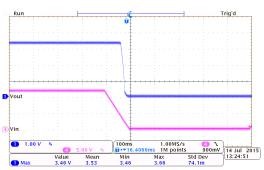
Power Off Response: HT7333-2 (I<sub>OUT</sub>=250mA, T<sub>FALL</sub>=100ms)
