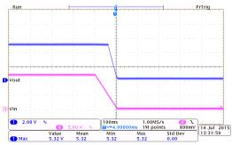
Power Off Response: HT7350-2 (I<sub>OUT</sub>=0mA, T<sub>FALL</sub>=100ms)
