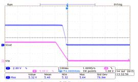
Power Off Response: HT7350-2 (I<sub>OUT</sub>=250mA, T<sub>FALL</sub>=100ms)
