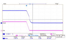
Power Off Response: HT7333-2 (I<sub>OUT</sub>=250mA, T<sub>FALL</sub>=0.1ms)
