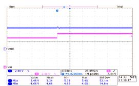
Line Trasient Response: HT7350-2 (I<sub>OUT</sub>=10mA)
