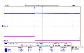
Load Transient Response: HT7350-2 ( $V_{\text{IN}}$ =7.0V,  $I_{\text{OUT}}$ =40mA to 0mA)
