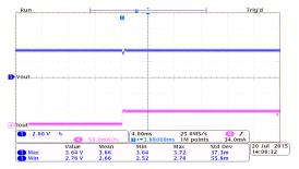
Load Transient Response: HT7333-2 ( $V_{\text{IN}}$ =5.3V,  $I_{\text{OUT}}$ =0mA to 40mA)
