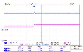
Line Trasient Response: HT7333-2 (I<sub>OUT</sub>=10mA)
