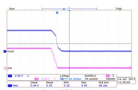
Power Off Response: HT7350-2 (I<sub>OUT</sub>=250mA, T<sub>FALL</sub>=0.1ms)
