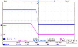
Power Off Response: HT7333-2 (I<sub>OUT</sub>=0mA, T<sub>FALL</sub>=100ms)
