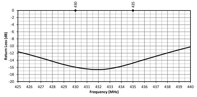
Figure 6. ANT-433-WRT Return Loss, Free SpacePlane
