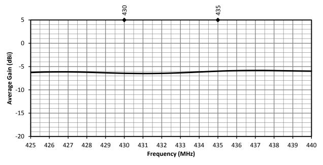
Figure 15. ANT-5GW-MMG1-SMA Antenna Average Gain, Free Space
