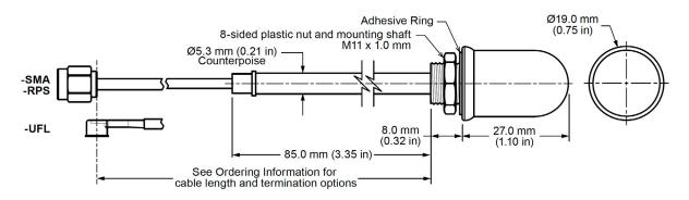
Figure 1. ANT-433-WRT Antenna Dimensions
