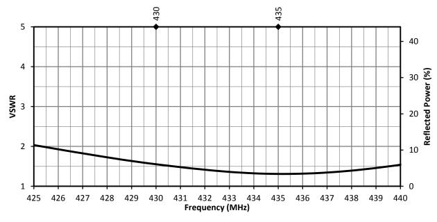
Figure 12. ANT-433-WRT VSWR, at Center of Ground Plane
