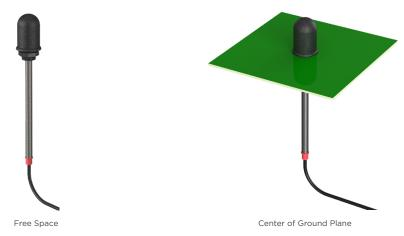
Figure 3. ANT-433-WRT Test Orientations
