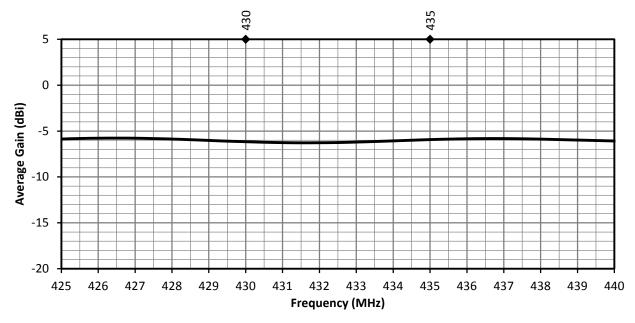
Figure 8. ANT-5GW-MMG1-SMA Antenna Average Gain on Ground Plane
