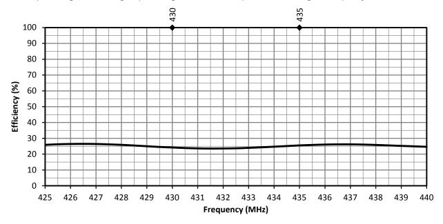
Figure 9. ANT-433-WRT Antenna Radiation Efficiency, Free Space
