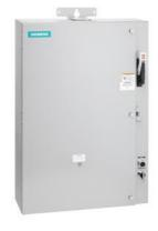
Pump control panel, Size 3, Three phase full voltage, Solid-state overload relay, OLR amp range 25-100A, 220-240/440-480VAC 60Hz coil, Standard type contactor, 100A fusible disconnect, 100A/600V fuse clip, HOA Sel Sw. <(>&<)> Start P.B., Enclosure NEMA type 3/3R, Weather proof outdoor use
