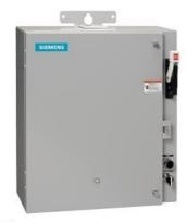
Pump control panel, Size 2, Three phase full voltage, Solid-state overload relay, OLR amp range 13-52A, 190-220/220-240V 50/60Hz coil, Standard type contactor, 50A circuit breaker, HOA Sel Sw. <(>&<)> Start P.B., Enclosure NEMA type 3/3R, Weather proof outdoor use
