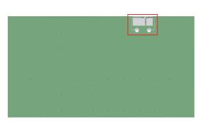
PCB size: 120mm x 65mm x 1mm Antenna area: 13 x 6 mm
