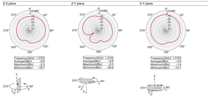
Tested antenna has been soldered. Evaluation board size is 120×65×1 mm.
