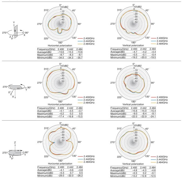
• Tested antenna has been soldered. Evaluation board size is 120×65×1 mm.
