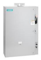
Pump control panel, Size 4, Three phase full voltage, Solid-state overload relay, OLR amp range 50-200A, 110-120/220-240VAC 60Hz coil, Standard type contactor, 200A fusible disconnect, 200A/600V fuse clip, HOA Sel Sw. <(>&<)> Start P.B., Enclosure NEMA type 3/3R, Weather proof outdoor use
